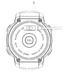
Please note that the two contacts of the charging cable can not touch the conductive object at the same time, otherwise it will cause short circuit combustion.
